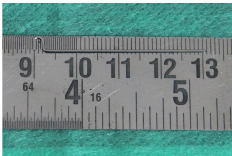
**Figure 2** The u-shaped bend. U-shaped bend with 2-mm separation between the limb and 90° vertical bend given to the 'u' bend.
