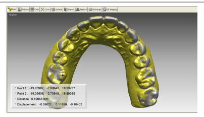
**Fig. 2** Discrepancies in the three-dimensional direction were calculated in the incisor and molar regions. Three reference points were selected, and the point-to-point distance between each point on the intraoral scan and the corresponding model scan was computed. The point-to-point distance was regarded as the displacement of the intraoral scan to the model scan, and the relative distance was calculated
