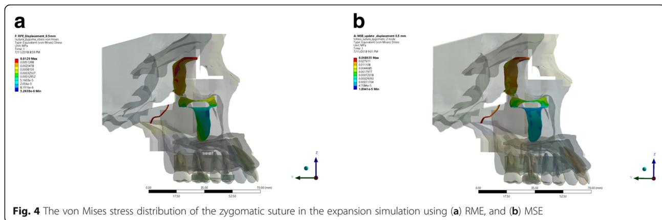
**Fig. 4** The von Mises stress distribution of the zygomatic suture in the expansion simulation using (a) RME, and (b) MSE
