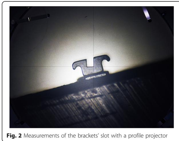
**Fig. 2** Measurements of the brackets’ slot with a profile projector
