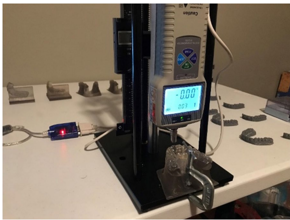
Fig. 3 Experimental Test Stand with dynamometer and integrated caliper prior to initializing displacement test of TFA aligner on the test model
