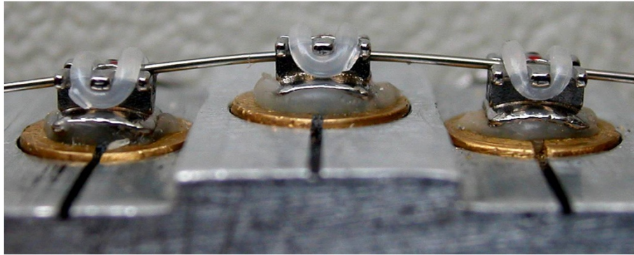
Figure 2 Stainless steel support of the horizontal bracket displacement experimental model. The central bracket is 1 mm buccally displaced relative to the adjacent brackets.
