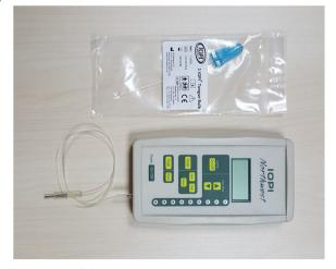
Fig. 1 Iowa Oral Pressure Instrument
